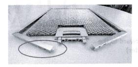
Place the cutted new filter mat carefully into the frame.
