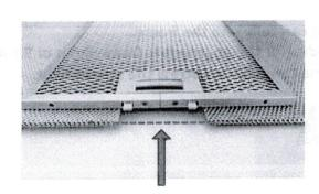
Mark the filter size on the new expanded metal layer.
